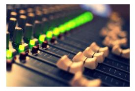
At the heart of every sound system is the mixer (also sometimes referred to as a "mixing board", "board", "desk", or "mixing console"). This device serves as the primary control center for the sound system, so it's important to have a clear understanding of how things work, and the "ins and outs" of working with a mixer.
